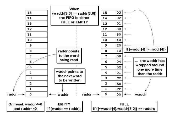
Figure 1 - FIFO full and empty conditions
