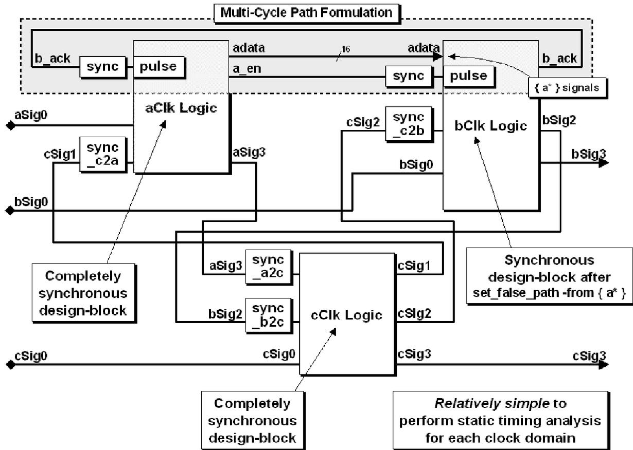
Figure 31 - Partitioned design with MCP formulation
