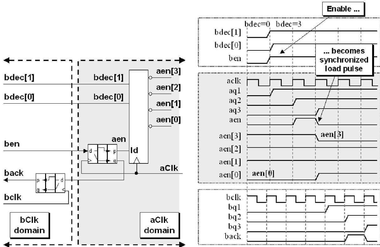
Figure 17 - Logic to pass a synchronized enable pulse between clock domains
