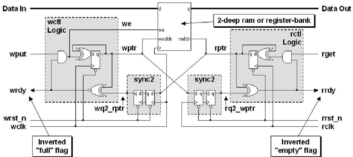
Figure 29 - 1-deep / 2-register FIFO synchronizer block diagram
