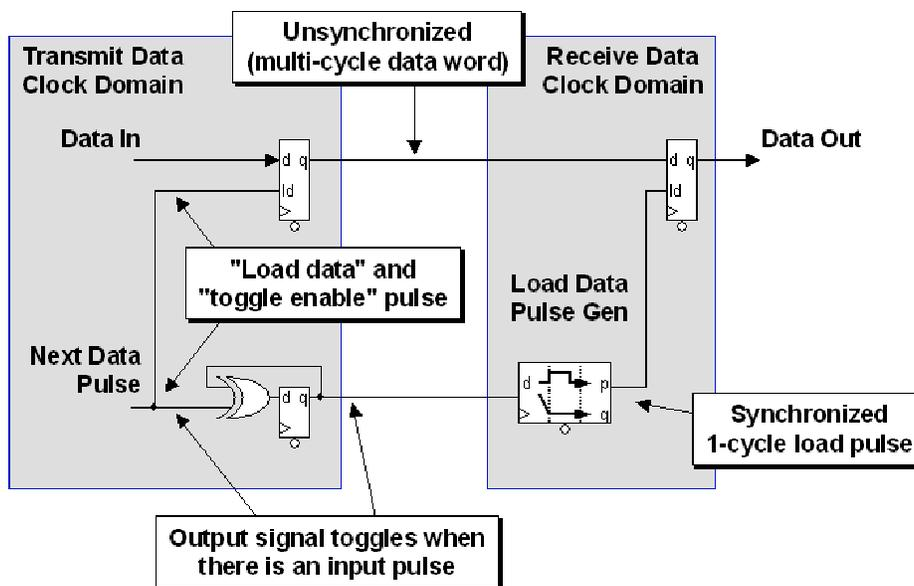
Figure 20 - Multi-Cycle Path (MCP) formulation toggle-pulse generation
