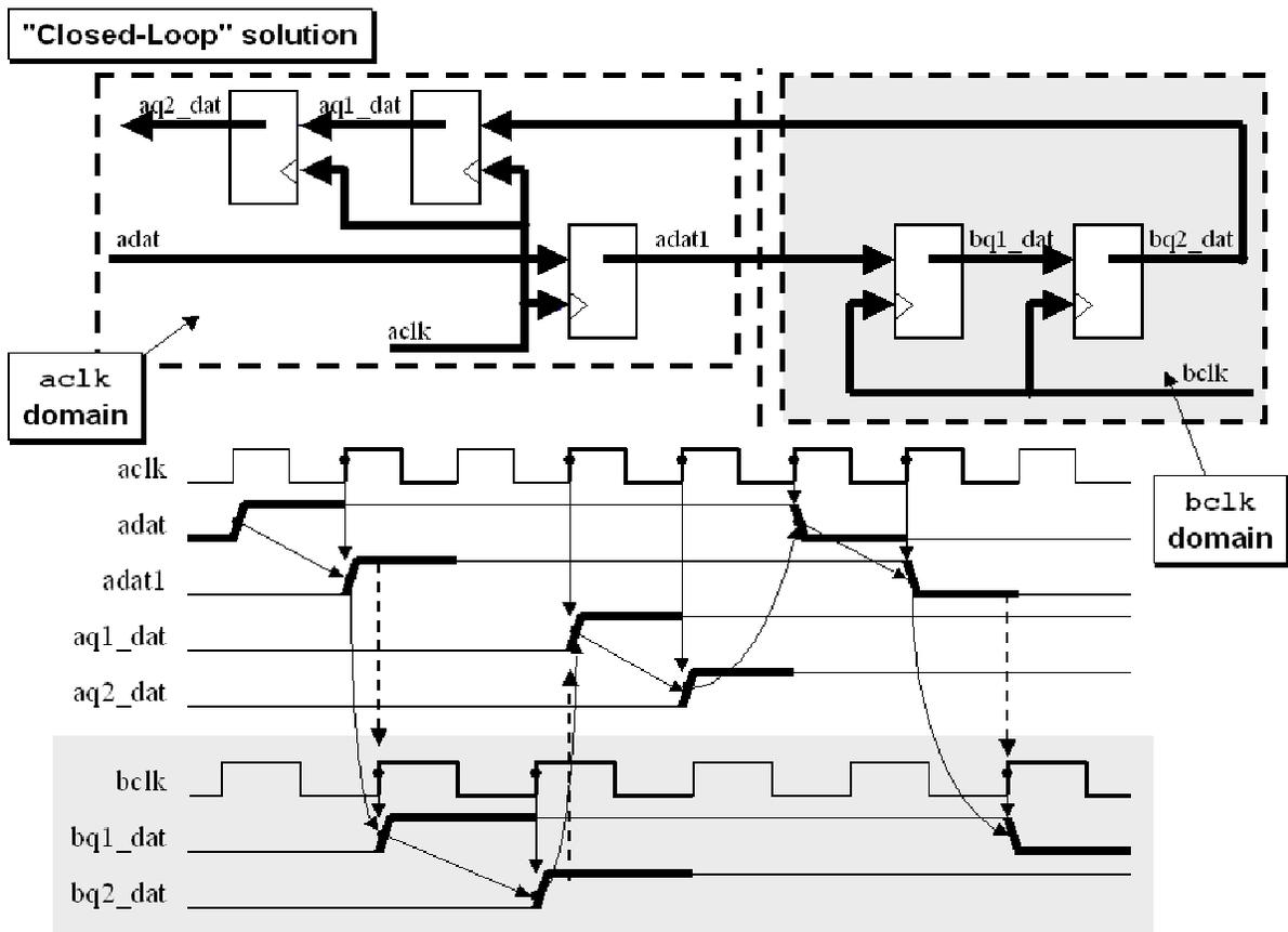
Figure 11 - Signal with feedback to acknowledge receipt
