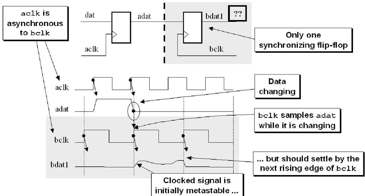
Figure 1 - Asynchronous clocks and synchronization failure
