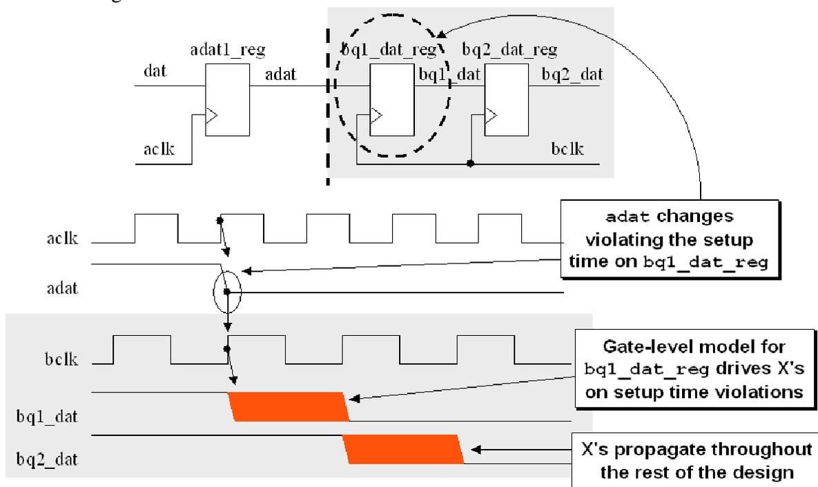
Figure 32 - Synchronizer gate-level CDC simulation waveforms
