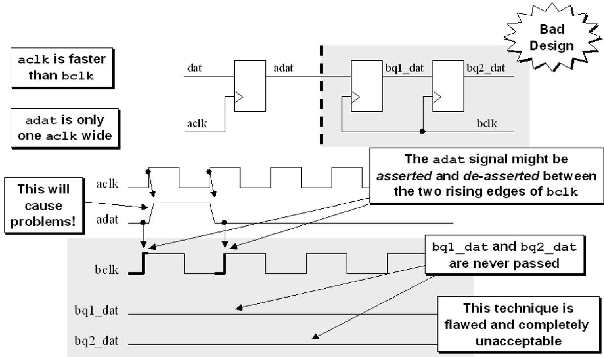
Figure 8 - Short CDC signal pulse missed during synchronization
