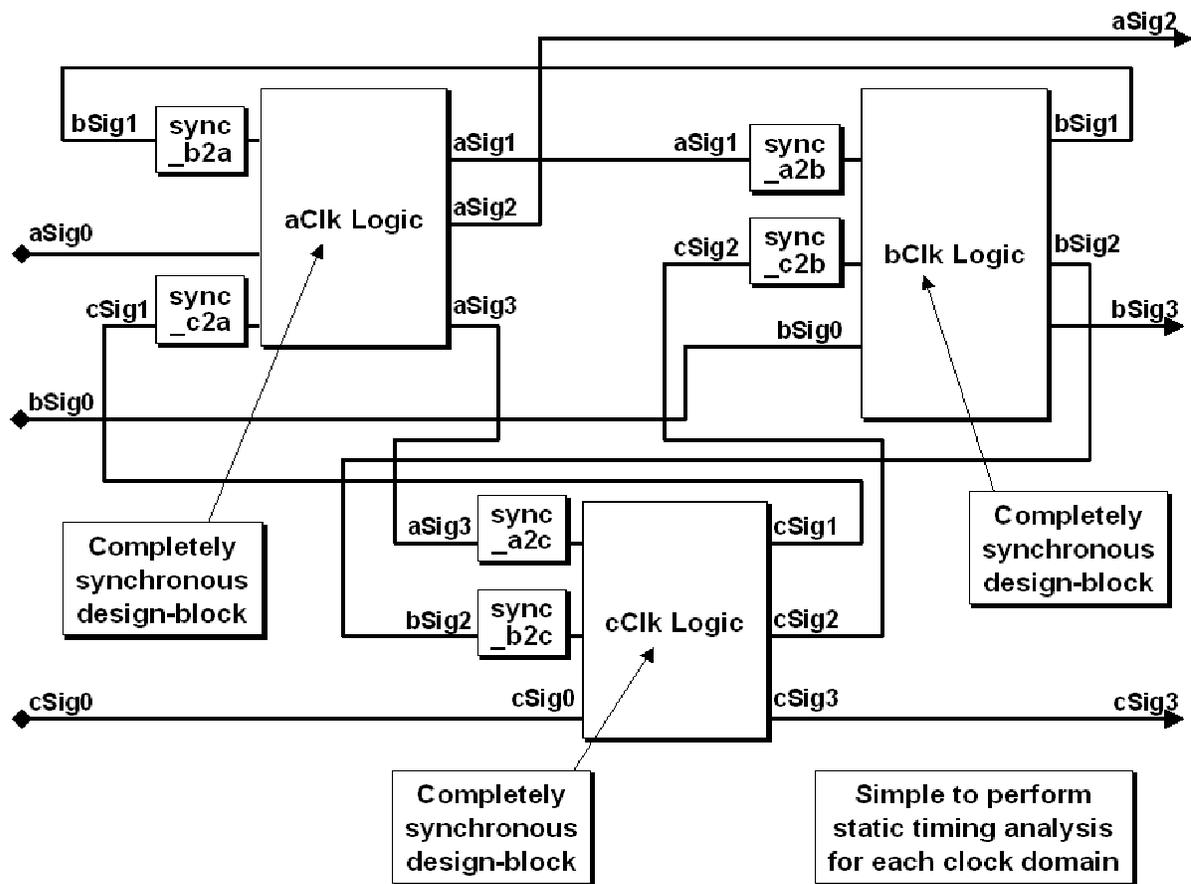
Figure 30 - Design partitioned on clock boundaries
